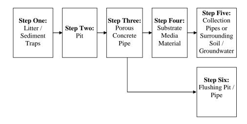
Figure 1. The Exfiltration Stormwater Treatment Process
