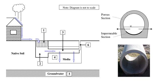
Figure 2. The Exfiltration Stormwater Treatment System and Porous Pipe
