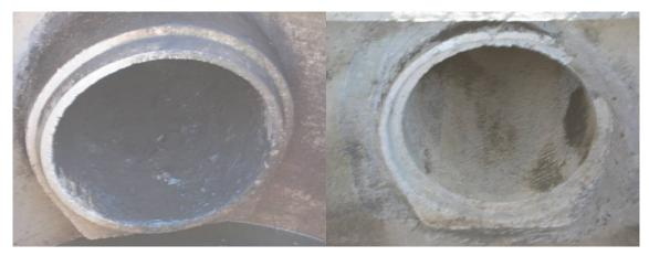
Figure 5. Porous Concrete Pipe – Before (Left) and After (Right) Cleaning
