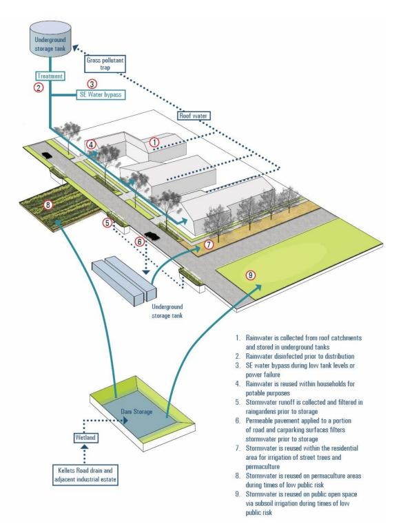
Figure 1 Schematic of the proposed Integrated Water Cycle Management at Stamford Park
