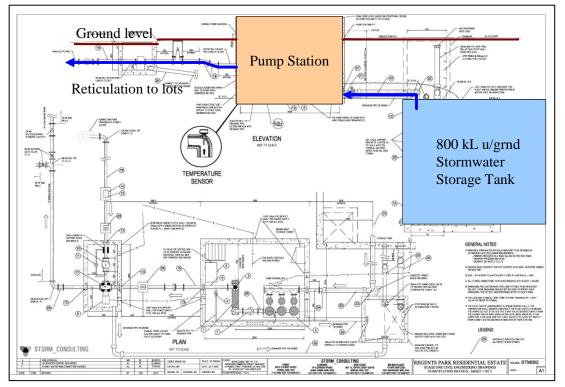
Figure 4 Pump station, UV disinfection and automated valve box
