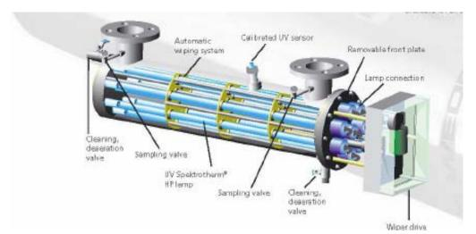
Figure 3 Self cleansing UV disinfection unit used at Ashgrove Estate.
