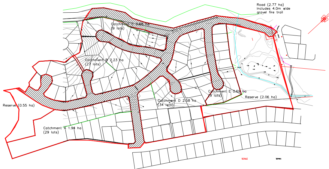
Figure 1: Fictitious subdivision that forms the basis of the case study for modelling purposes
