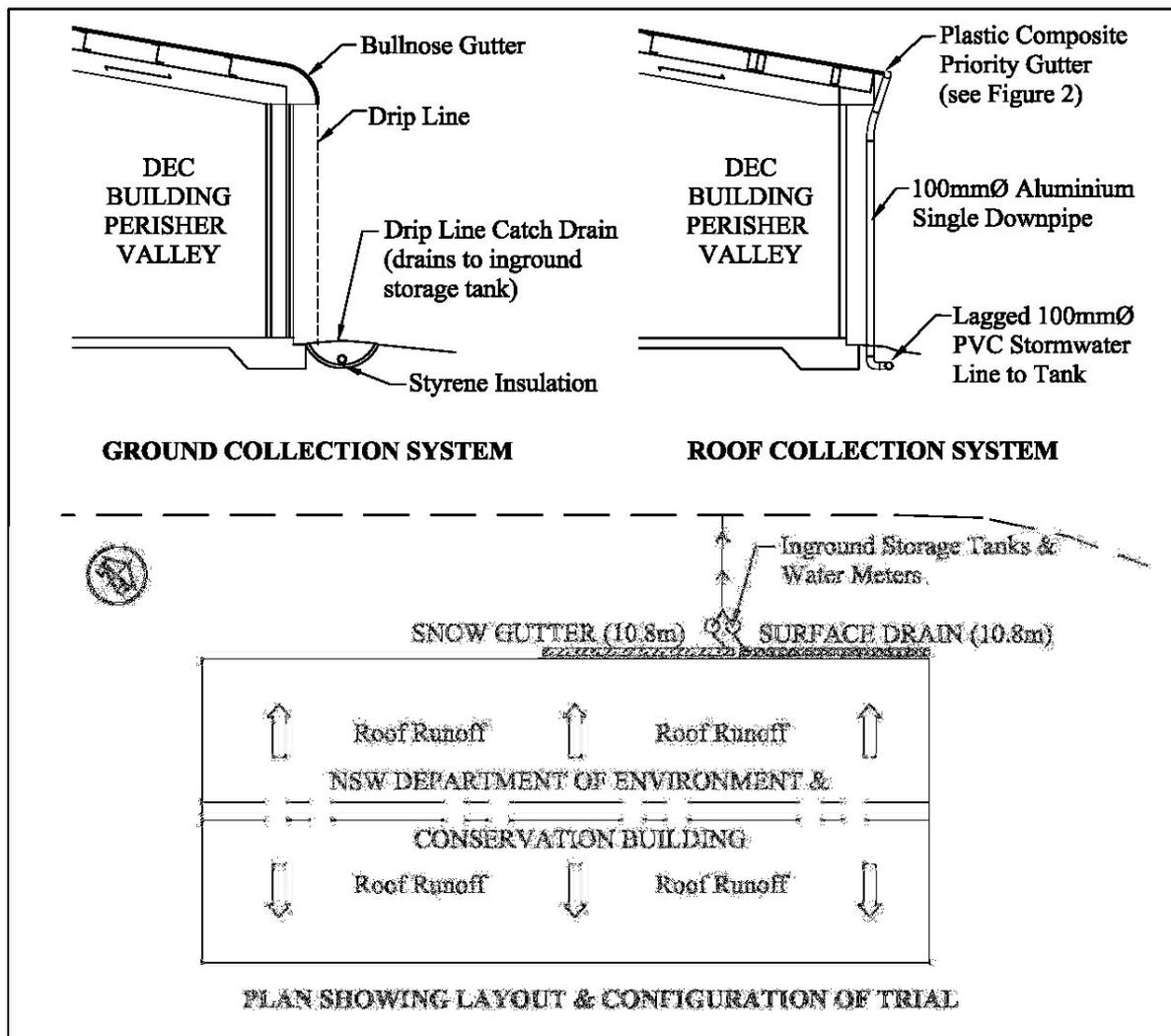
**Figure 1.** Location and configuration of the roof water harvesting trial at Perisher Valley (1,720m ASL).
